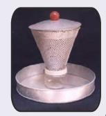
fixed at the bottom with a container and circular dish, which are to be smeared with sticky material like vaseline. Farmers, before storing their pulses, should take 200 g of pulses to be stored and put them in the cup. When the field carried
